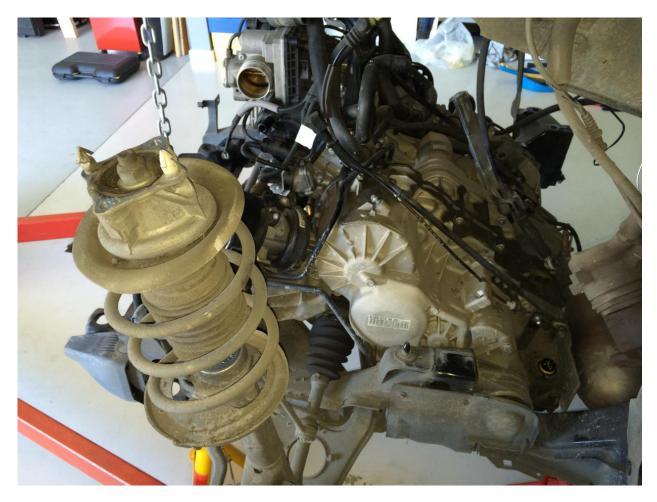
With the body fully raised you are pretty much in a position to jack the motor/transmission/subframe down onto a dolly to move it clear of the body. I used my own dolly made previously using 3 pieces of 20mm particle board and 150kg rated castors (see photo below). I was able to balance the entire assembly on the dolly and move it as a complete unit.
